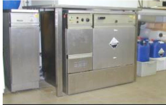
Caustic Wash / Pasteurizer
